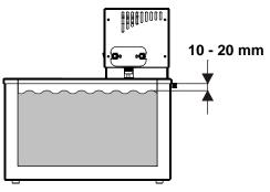
In no case the fluid level may be lower than 60 mm under the edge. This can cause severe damage to the heating element.
